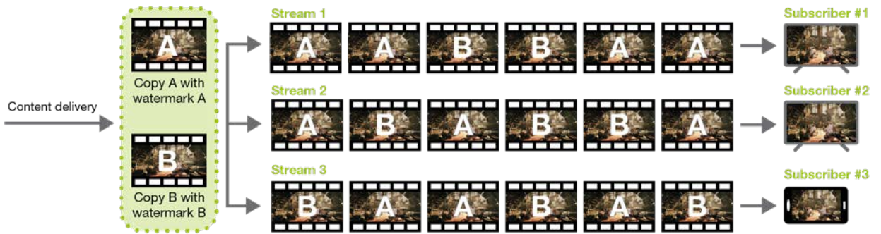
A/B Variant watermarking interleaves video segments from two copies of a stream to create a unique watermark pattern
