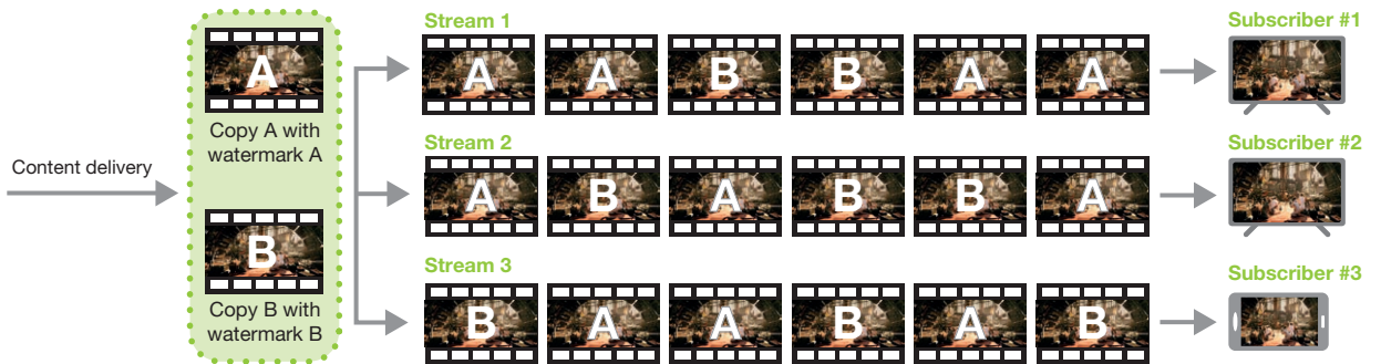
A/B Variant watermarking interleaves video segments from two copies of a stream to create a unique watermark pattern
